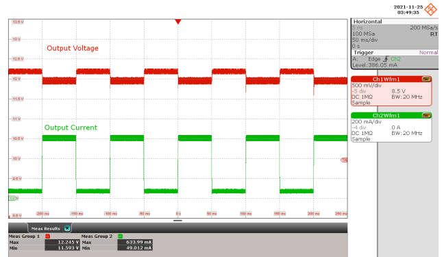
Figure 98 – Transient Output Waveforms. 230 VAC. Output Voltage: 500 mV / div., 50 ms / div. Output Current: 200 mA / div., 50 ms / div. Load Transient: 10 % - 100%. Duty Cycle, Slew Rate: 50%, 0.8 A / \mu s. Frequency: 10 Hz. V_{MAX} : 12.245 V, V_{MIN} : 11.593 V.
