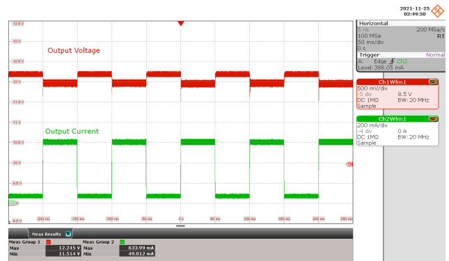
Figure 98 – Transient Output Waveforms. 230 VAC. Output Voltage: 500 mV / div., 50 ms / div. Output Current: 200 mA / div., 50 ms / div. Load Transient: 10 % - 100%. Duty Cycle, Slew Rate: 50%, 0.8 A / \mu s. Frequency: 10 Hz. V_{MAX} : 12.245 V, V_{MIN} : 11.593 V.
