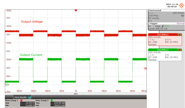
Figure 96 – Transient Output Waveforms. 115 VAC. Output Voltage: 500 mV / div., 50 ms / div. Output Current: 200 mA / div., 50 ms / div. Load Transient: 10 % - 100%. Duty Cycle, Slew Rate: 50%, 0.8 A / \mu s. Frequency: 10 Hz. V_{MAX} : 12.245 V, V_{MIN} : 11.692 V.
