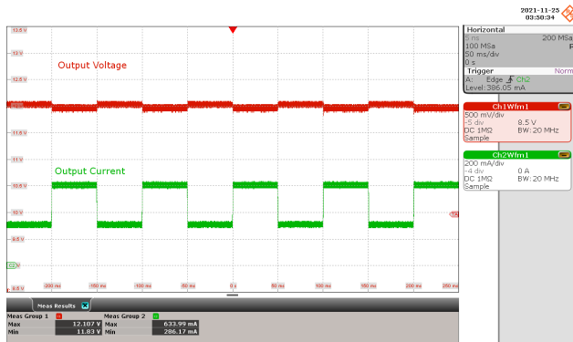
Figure 93 – Transient Output Waveforms. 85 VAC. Output Voltage: 500 mV / div., 50 ms / div. Output Current: 200 mA / div., 50 ms / div. Load Transient: 50 % - 100%. Duty Cycle, Slew Rate: 50%, 0.8 A / \mu s. Frequency: 10 Hz. V_{MAX} : 12.107 V, V_{MIN} : 11.83 V.
