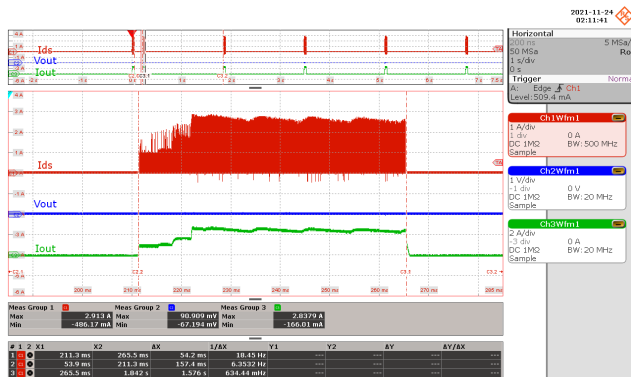
Figure 40 – Drain Current and Output Waveforms. 85 VAC Input. Drain Current: 1 A / div., 1 s / div. Output Voltage: 1 V / div., 1 s / div. Output Current: 2 A / div, 1 s / div. Zoom = 10 ms / div.
