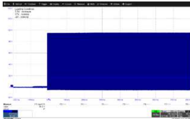
Figure 67 – Input: 530 VDC; 7.5 V Load: 65 mA; 17 V and -4 V Load: 120 mA.
