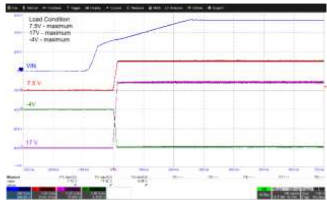
Figure 32 – Input: 530 VDC; 7.5 V Load: 1.3 A; 17 V and -4 V Load: 140 mA.
