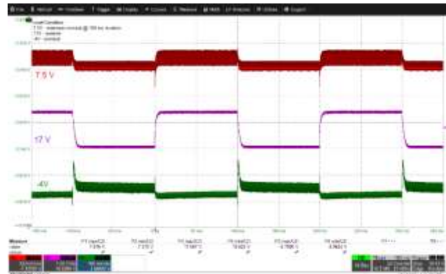
Figure 46 – Input: 375 VDC; 17 V and -4 V Load: 120 mA; 7.5 V Load: 65 mA – 1.13 A @ 100 ms duration with 100 ms / \mu A slew rate.
