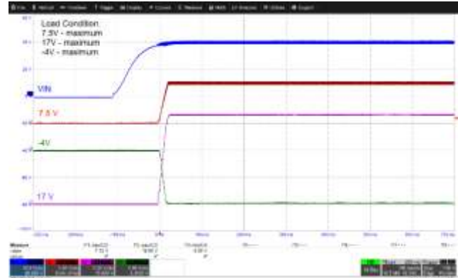
Figure 26 – Input: 40 VDC; 7.5 V Load: 1.3 A; 17 V and -4 V Load: 140 mA.
