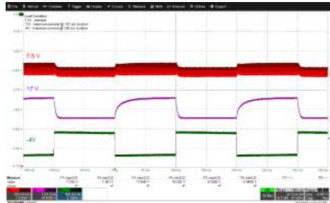
Figure 34 – Input: 40 VDC; 7.5 V Load: 1.13 A; 17 V and -4 V Load: 20 mA – 120 mA @ 100 ms duration with 100 ms / \mu A slew rate.
