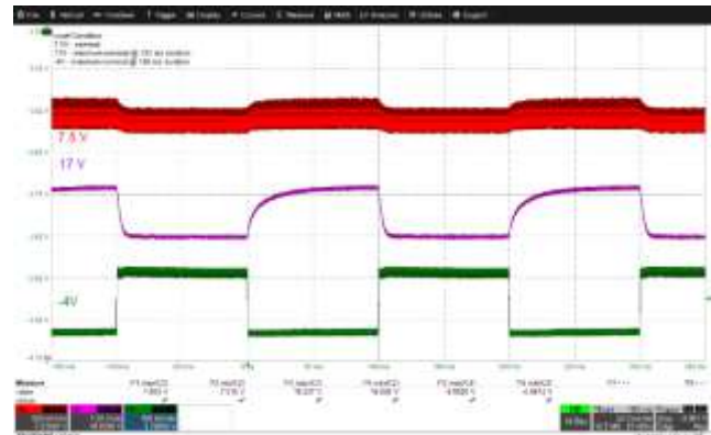
Figure 38 – Input: 375 VDC; 7.5 V Load: 1.13 A; 17 V and -4 V Load: 20 mA – 120 mA @ 100 ms duration with 100 ms / \mu A slew rate.
