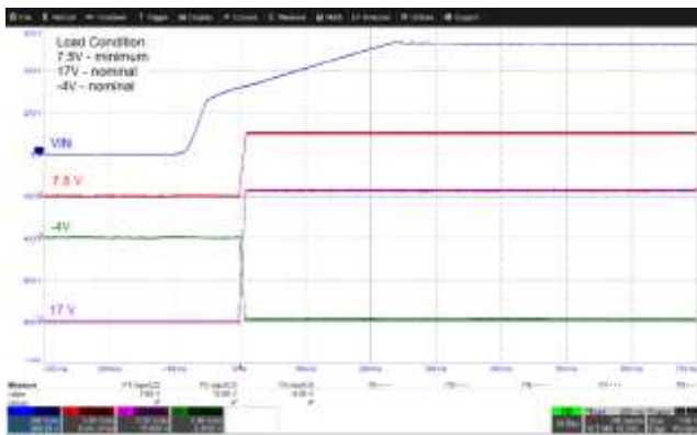
Figure 31 – Input: 530 VDC; 7.5 V Load: 65 mA; 17 V and -4 V Load: 120 mA.
