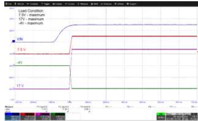
Figure 28 – Input: 300 VDC; 7.5 V Load: 1.3 A; 17 V and -4 V Load: 140 mA.
