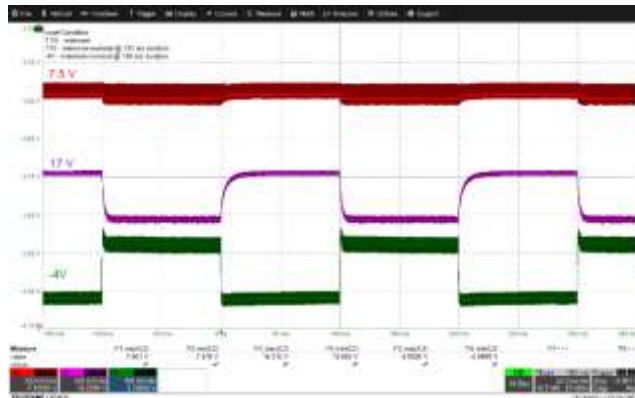
Figure 39 – Input: 530 VDC; 7.5 V Load: 65 mA; 17 V and -4 V Load: 20 mA – 120 mA @ 100 ms duration with 100 ms / \mu A slew rate.
