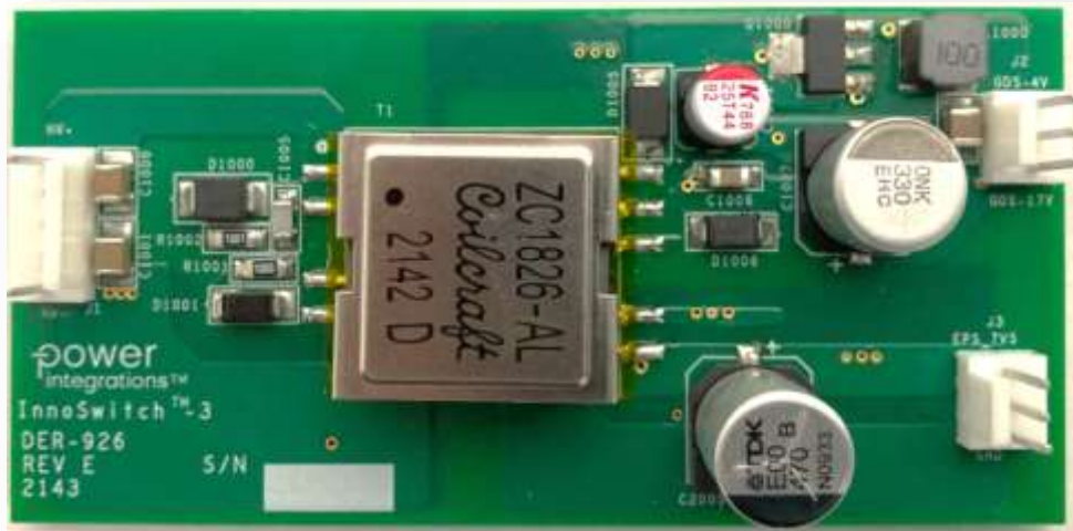
Figure 1 – Populated Circuit Board Photograph (88 mm x 43 mm), Top.
