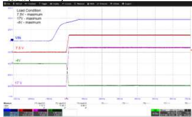
Figure 30 – Input: 375 VDC; 7.5 V Load: 1.3 A; 17 V and -4 V Load: 140 mA.
