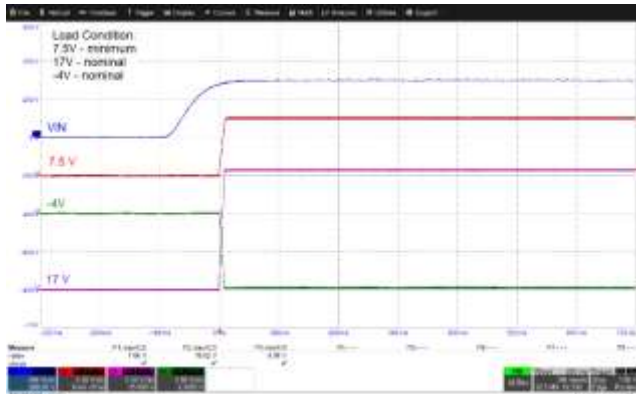
Figure 27 – Input: 300 VDC; 7.5 V Load: 65 mA; 17 V and -4 V Load: 120 mA.
