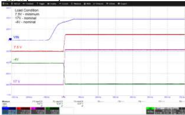
Figure 29 – Input: 375 VDC; 7.5 V Load: 65 mA; 17 V and -4 V Load: 120 mA.
