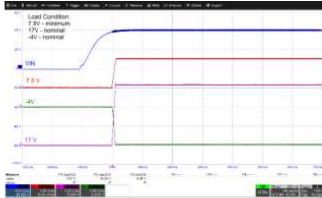
Figure 25 – Input: 40 VDC; 7.5 V Load: 65 mA; 17 V and -4 V Load: 120 mA.
