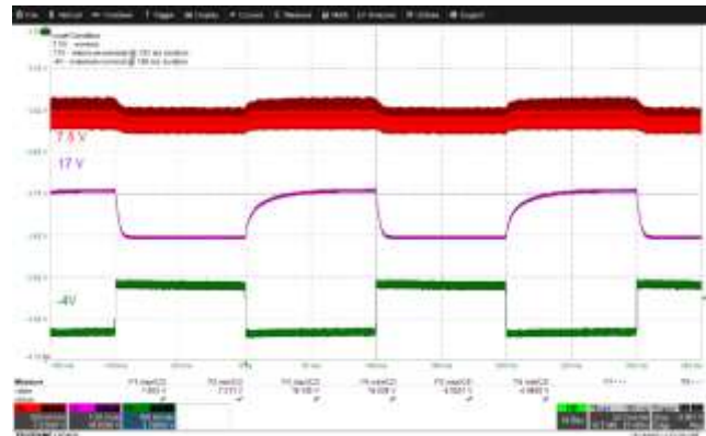
Figure 36 – Input: 300 VDC; 7.5 V Load: 1.13 A; 17 V and -4 V Load: 20 mA – 120 mA @ 100 ms duration with 100 ms / \mu A slew rate.
