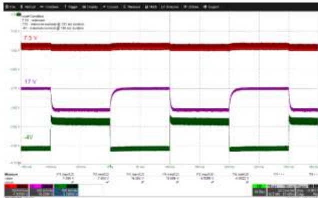
Figure 37 – Input: 375 VDC; 7.5 V Load: 65 mA; 17 V and -4 V Load: 20 mA – 120 mA @ 100 ms duration with 100 ms / \mu A slew rate.
