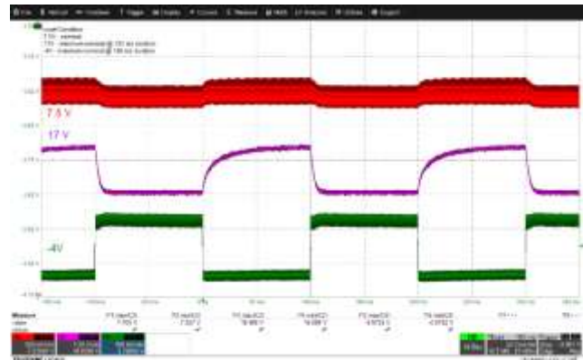
Figure 40 – Input: 530 VDC; 7.5 V Load: 1.13 A; 17 V and -4 V Load: 20 mA – 120 mA @ 100 ms duration with 100 ms / \mu A slew rate.
