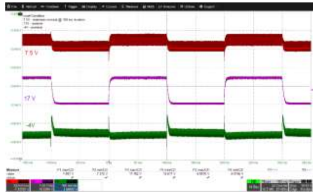
Figure 48 – Input: 530 VDC; 17 V and -4 V Load: 120 mA; 7.5 V Load: 65 mA – 1.13 A @ 100 ms duration with 100 ms / \mu A slew rate.
