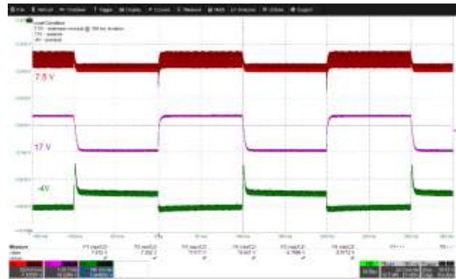
Figure 44 – Input: 300 VDC; 17 V and -4 V Load: 120 mA; 7.5 V Load: 65 mA – 1.13 A @ 100 ms duration with 100 ms / \mu A slew rate.
