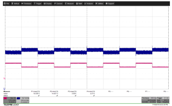
Figure 71 – Transient Response. 265 VAC, 15 V, 2.25 – 3 A Load Step. V_{MIN} : 14.831 V, V_{MAX} : 15.039 V. Upper: V_{OUT} , .2 V / div., 50 ms / div. Lower: I_{LOAD} , 2 A / div.
