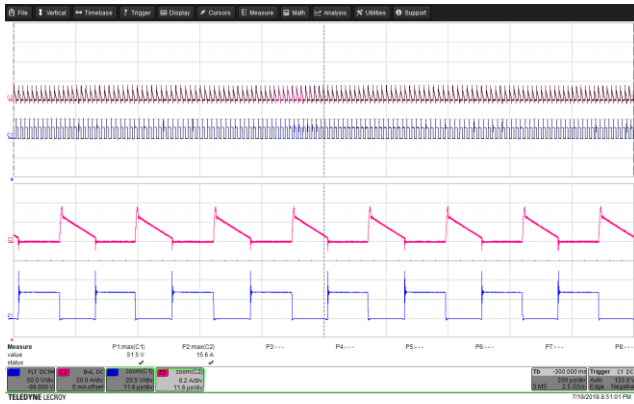
Figure 92 – SR FET Voltage Waveforms. 85 VAC, 15.0 V, 3 A Load (51.5 V MAX ). Upper: V DRAIN , 50 V, 200 μs / div. Lower: I DRAIN , 10 A / div.
