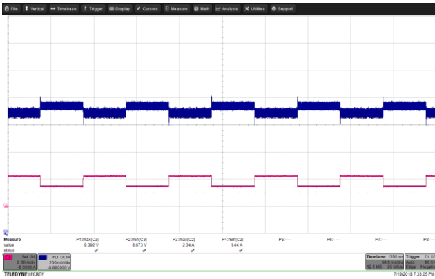
Figure 60 – Transient Response. 85 VAC, 9.0 V, 1.5 – 2.25 A Load Step. V_{MIN} : 8.873 V, V_{MAX} : 9.092 V. Upper: V_{OUT} , 0.2 V / div., 50 ms / div. Lower: I_{LOAD} , 2 A / div.
