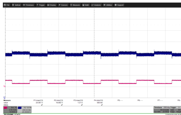
Figure 75 – Transient Response. 265 VAC, 20.0 V, 0.56 – 1.125 A Load Step. V_{MIN} 19.893 V, V_{MAX} : 20.061 V. Upper: V_{OUT} , 0.2 V / div., 50 ms / div. Lower: I_{LOAD} , 2 A / div.
