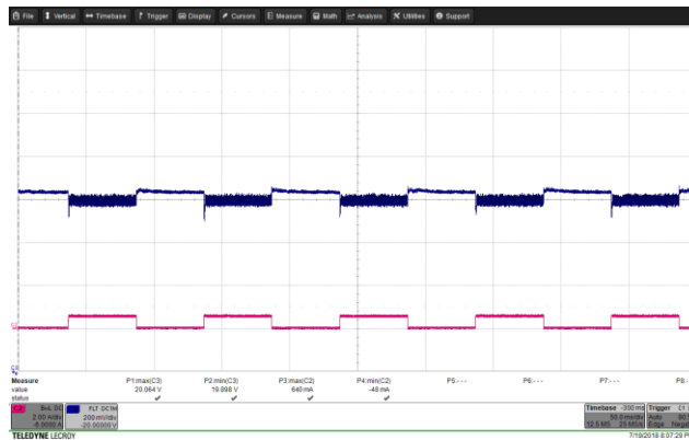
Figure 73 – Transient Response. 265 VAC, 20.0 V, 0 – 0.56 A Load Step. V_{MIN} 19.898 V, V_{MAX} : 20.064 V. Upper: V_{OUT} , 0.2 V / div., 50 ms / div. Lower: I_{LOAD} , 2 A / div.
