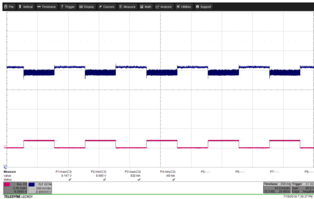
Figure 56 – Transient Response. 85 VAC, 9.0 V, 0 – 0.75 A Load Step. V_{MIN} 8.990 V, V_{MAX} : 9.147 V. Upper: V_{OUT} , 0.2 V / div., 50 ms / div. Lower: I_{LOAD} , 2 A / div.
