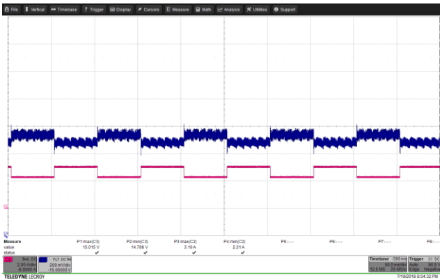
Figure 70 – Transient Response. 85 VAC, 15 V, 2.25 – 3 A Load Step. V_{MIN} : 14.786 V, V_{MAX} : 15.051 V. Upper: V_{OUT} , .2 V / div., 50 ms / div. Lower: I_{LOAD} , 2 A / div.
