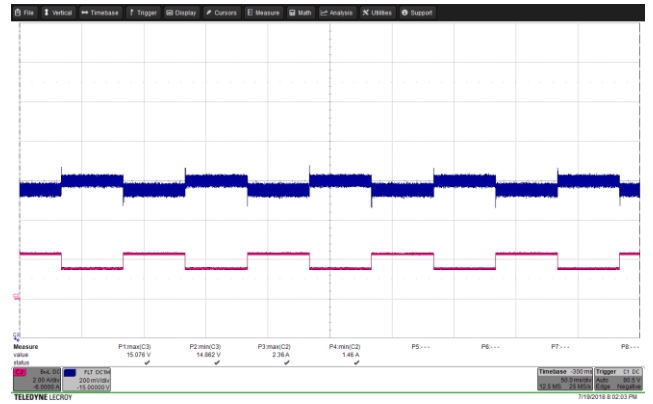
Figure 69 – Transient Response. 265 VAC, 15 V, 1.5 – 2.25 A Load Step. V_{MIN} : 14.862 V, V_{MAX} : 15.076 V. Upper: V_{OUT} , 0.2 V / div., 50 ms / div. Lower: I_{LOAD} , 2 A / div.
