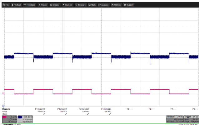
Figure 64 – Transient Response. 85 VAC, 15.0 V, 0 – 0.75 A Load Step. V_{MIN} 14.879 V, V_{MAX} : 15.092 V. Upper: V_{OUT} , 0.2 V / div., 50 ms / div. Lower: I_{LOAD} , 2 A / div.
