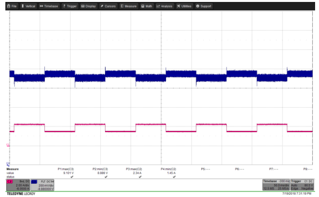
Figure 61 – Transient Response. 265 VAC, 9.0 V, 1.5 – 2.25 A Load Step. V_{MIN} : 8.886 V, V_{MAX} : 9.101 V. Upper: V_{OUT} , 0.2 V / div., 50 ms / div. Lower: I_{LOAD} , 2 A / div.
