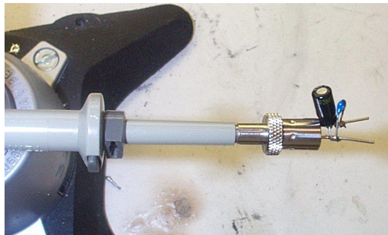
Figure 99 – Oscilloscope Probe with Probe Master ( www.probemaster.com ) 4987A BNC Adapter. (Modified with wires for ripple measurement, and two parallel decoupling capacitors added)
