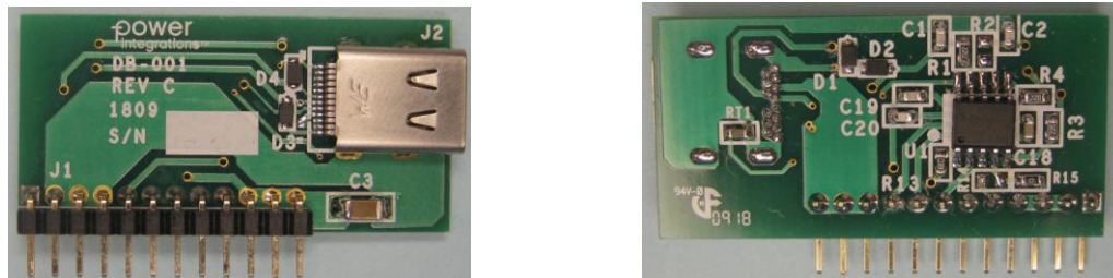
Figure 5 – Populated Circuit Board Photograph, Daughter Board [Front and Rear].
