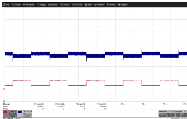
Figure 67 – Transient Response. 265 VAC, 15.0 V, 0.75 – 1.5 A Load Step. V_{MIN} 14.879 V, V_{MAX} : 15.088 V. Upper: V_{OUT} , 0.2 V / div., 50 ms / div. Lower: I_{LOAD} , 2 A / div.
