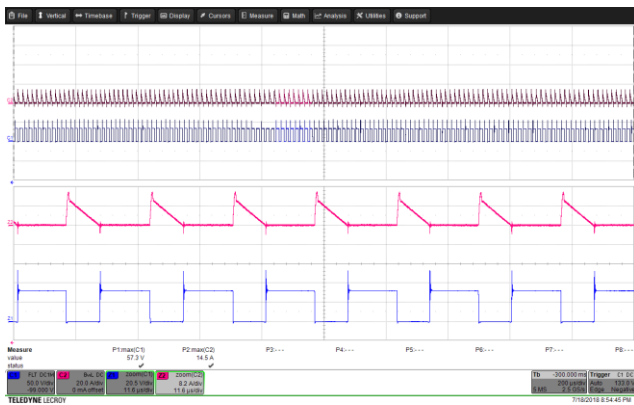
Figure 94 – SR FET Voltage Waveforms. 85 VAC, 20.0 V, 2.25 A Load (57.3 V MAX ). Upper: V DRAIN , 50 V, 200 μs / div. Lower: I DRAIN , 10 A / div.
