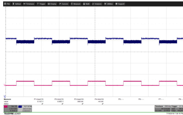
Figure 57 – Transient Response. 265 VAC, 9.0 V, 0 – 0.75 A Load Step. V_{MIN} 8.995 V, V_{MAX} : 9.143 V. Upper: V_{OUT} , 0.2 V / div., 50 ms / div. Lower: I_{LOAD} , 2 A / div.
