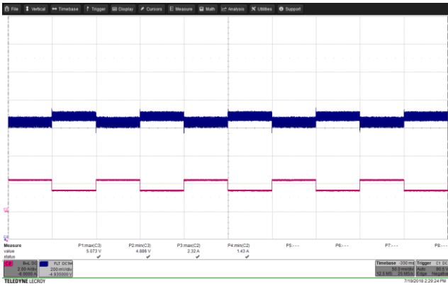
Figure 52 – Transient Response. 85 VAC, 5.0 V, 1.5 – 2.25 A Load Step. V_{MIN} : 4.886 V, V_{MAX} : 5.073 V. Upper: V_{OUT} , 0.2 V / div., 50 ms / div. Lower: I_{LOAD} , 2 A / div.
