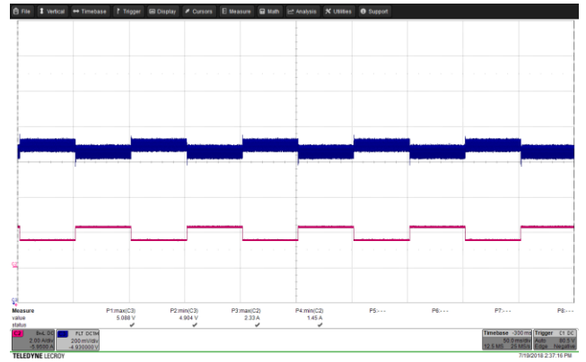
Figure 53 – Transient Response. 265 VAC, 5.0 V, 1.5 – 2.25 A Load Step. V_{MIN} : 4.904 V, V_{MAX} : 5.088 V. Upper: V_{OUT} , 0.2 V / div., 50 ms / div. Lower: I_{LOAD} , 2 A / div.
