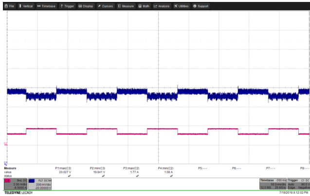
Figure 76 – Transient Response. 85 VAC, 20.0 V, 1.125 – 1.68 A Load Step. V_{MIN} : 19.841 V, V_{MAX} : 20.027 V. Upper: V_{OUT} , 0.2 V / div., 50 ms / div. Lower: I_{LOAD} , 2 A / div.
