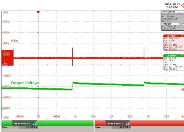
**Figure 77 – 90 VAC 60 Hz, No load**
