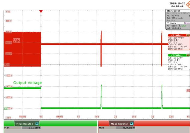
**Figure 76 – 265 VAC 60 Hz, Full load**
