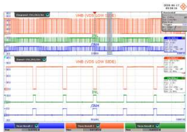
Figure 31 – INL and /INH Signal at 400 W Load. CH2: V_{HB\_PHASEW} , 100 V / div. CH4: V_{INL} , 5 V / div. CH1: V_{INH} , 5 V / div. Time Scale: 2 ms / div. Time Scale (Zoomed Area): 50 \mu s / div.
