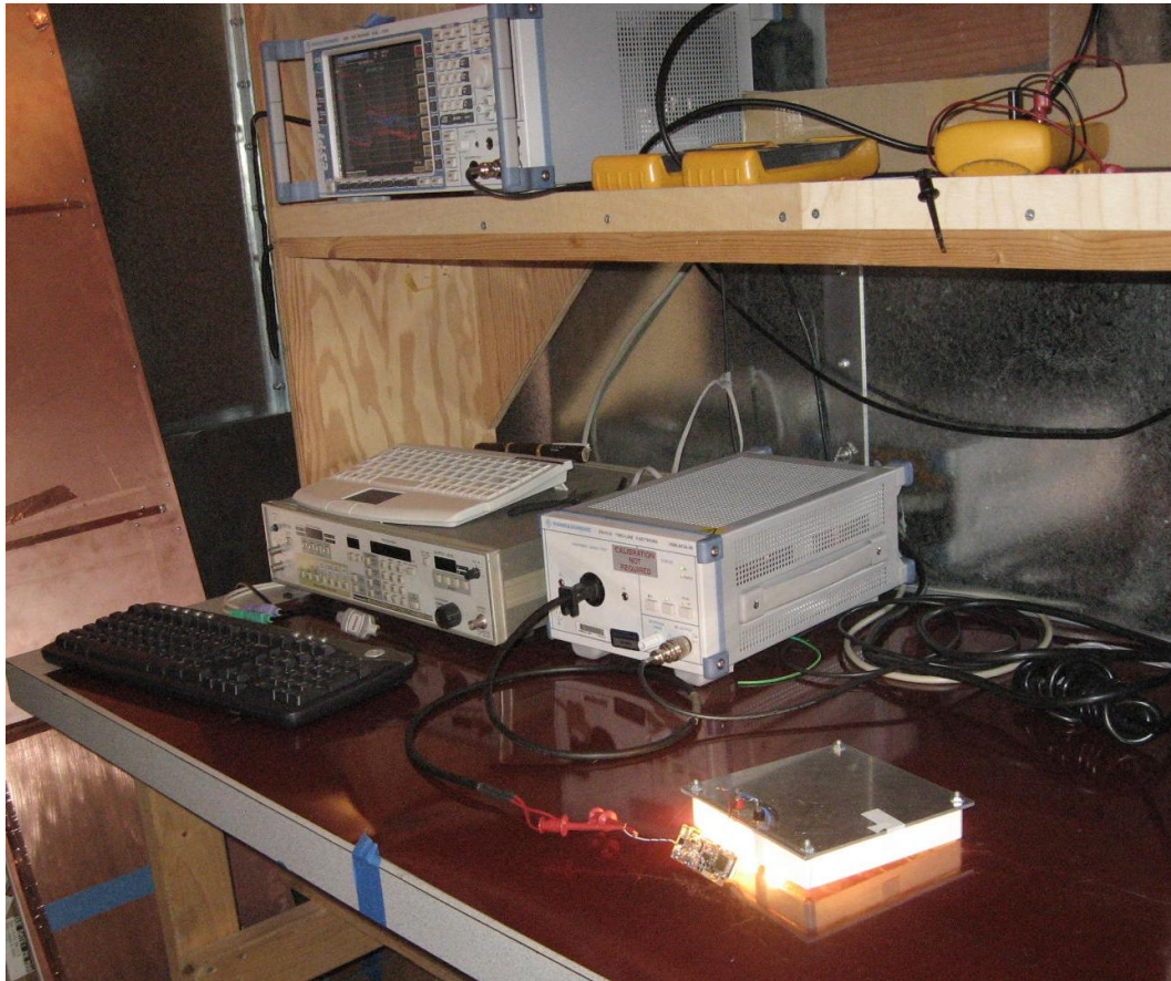
Figure 43 – Conducted Emissions Measurement Set-up.
