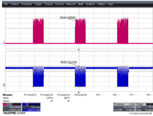
Figure 34 – 300 VAC 50 Hz, Output Short. Upper: I_{DRAIN} , 0.5 A / div. Lower: V_{DRAIN} , 100 V, 100 ms / div.
