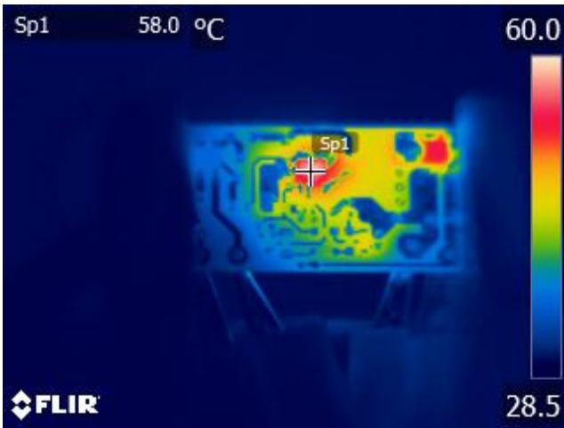
Figure 41 – LNK-XT2 (U1). Spot: 58.0 °C.
