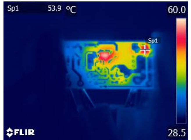
Figure 42 – Secondary Snubber Diode (D3). Spot: 53.9 °C.
