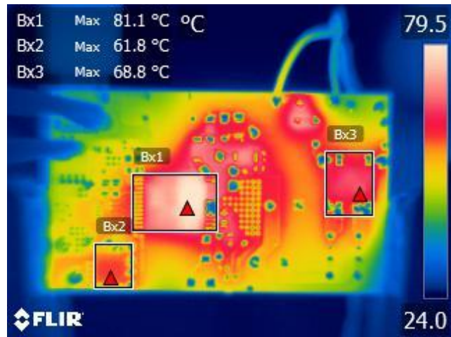
Figure 43 – Bottom Side Thermal Image. Bx1: InnoSwitch3-Pro = 81.1 °C. Bx2: SR FET = 61.8 °C. Bx3: Bridge Rectifier BR1 = 68.8 °C.
