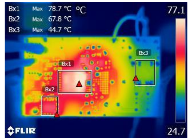
Figure 41 – Bottom Side Thermal Image. Bx1: InnoSwitch3-Pro = 78.7 °C. Bx2: SR FET = 67.8 °C. Bx3: Bridge Rectifier BR1 = 44.7 °C.
