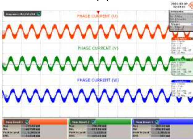
Figure 26 – Phase Current at 100 W Load. CH1: I_{PHASEU} , 1 A / div. CH2: I_{PHASEV} , 1 A / div. CH3: I_{PHASEW} , 1 A / div. Time Scale: 10 ms / div. RMS Current (U) = 314 mA RMS . RMS Current (V) = 325 mA RMS . RMS Current (W) = 307 mA RMS .
