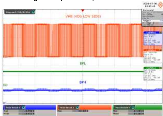
Figure 33 – BPL and BPH Signals at 30W Load.
