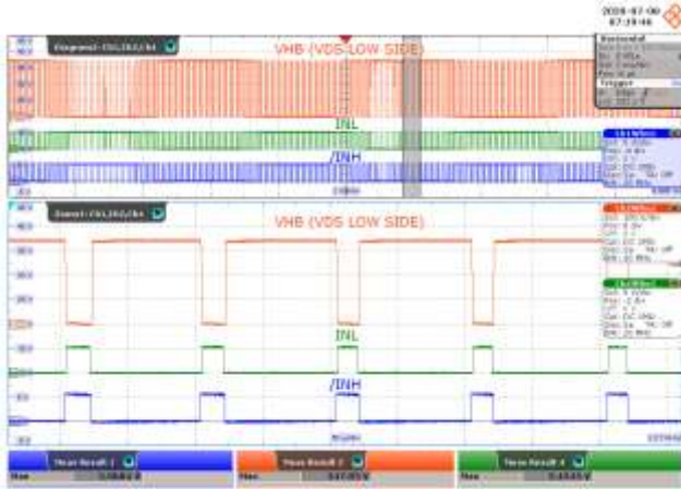
Figure 28 – INL and /INH Signal at Light Load. CH2: V_{HB\_PHASEW} , 100 V / div. CH4: V_{INL} , 5 V / div. CH1: V_{INH} , 5 V / div. Time Scale: 2 ms / div. Time Scale (Zoomed Area): 50 \mu s / div.
