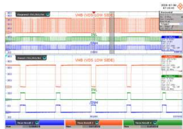
Figure 31 – INL and /INH Signal at 200 W Load. CH2: V_{HB\_PHASEW} , 100 V / div. CH4: V_{INL} , 5 V / div. CH1: V_{INH} , 5 V / div. Time Scale: 2 ms / div. Time Scale (Zoomed Area): 50 \mu s / div.
