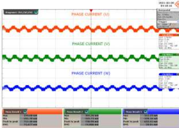
Figure 24 – Phase Current at Light Load. CH1: I_{PHASEU} , 1 A / div. CH2: I_{PHASEV} , 1 A / div. CH3: I_{PHASEW} , 1 A / div. Time Scale: 10 ms / div. RMS Current (U) = 72 mA RMS . RMS Current (V) = 74 mA RMS . RMS Current (W) = 60 mA RMS .
