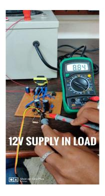
There is an instability in +12V-1A output of SMPS, even though +5V-1A is stable in both load and no-load conditions. Changing the value of bulk capacitor and pi inductor value at output had no significant improvement.
