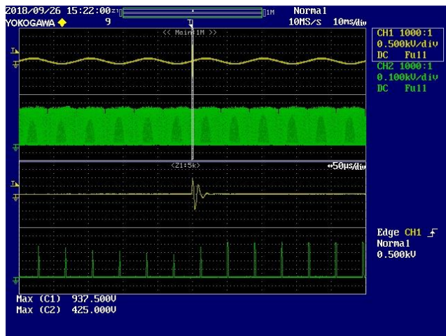
Figure 140 – (+) 2.5 kV Ring Wave Surge, 0° Phase Angle. Lower: V_{DRAIN} , 100 V / div., 10 ms / div. Peak V_{DRAIN} : 425 V.
