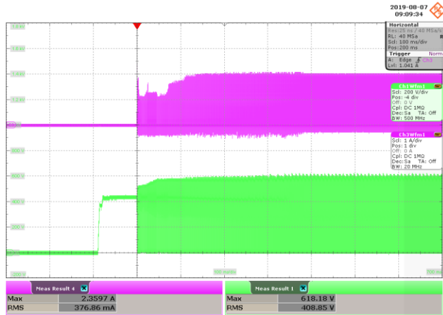
Figure 93 – 305 VAC, 48 V LED Load. Upper: I_{DRAIN} , 1 A / div. Lower: V_{DRAIN} , 200 V / div., 100 ms / div.
